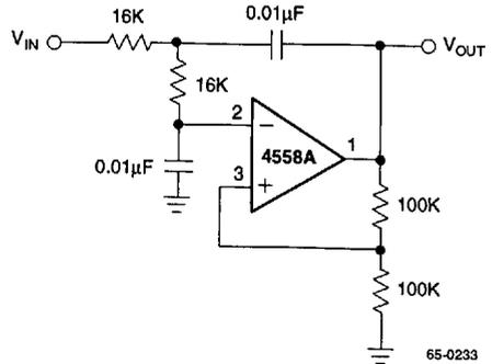
Figure 23. DC Coupled 1kHz Low-Pass Active Filter
