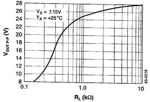
Figure 8. Output Voltage Swing vs. Load Resistance
