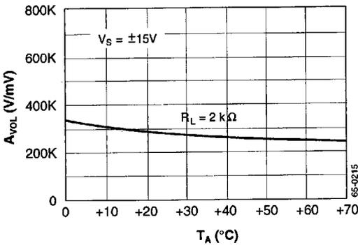
Figure 5. Open Loop Voltage Gain vs. Temperature
