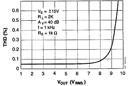
Figure 16. Total Harmonic Distortion vs. Output Voltage
