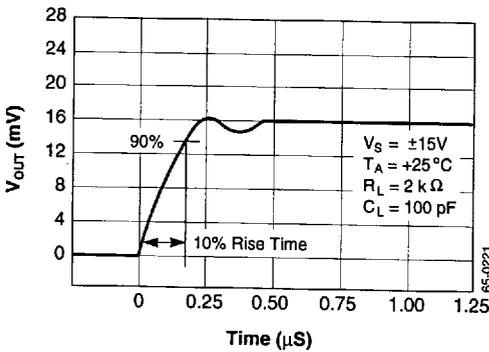
Figure 11. Transient Response Output Voltage vs. Time
