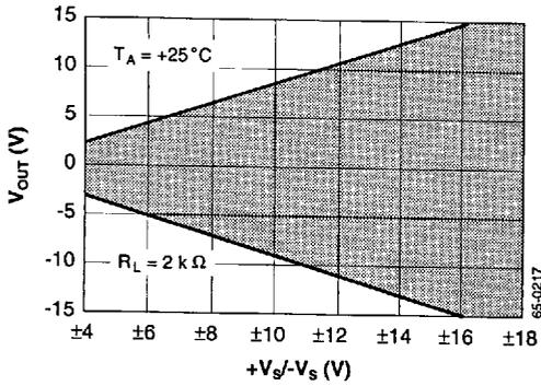
Figure 7. Output Voltage Swing vs. Supply Voltage
