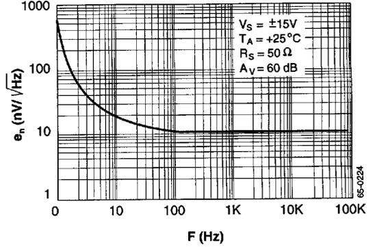
Figure 14. Input Noise Voltage Density vs. Frequency
