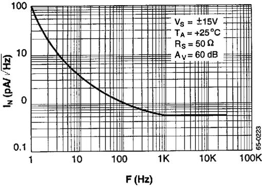
Figure 13. Input Noise Current Density vs. Frequency
