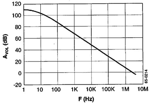
Figure 4. Open Loop Voltage Gain vs. Frequency
