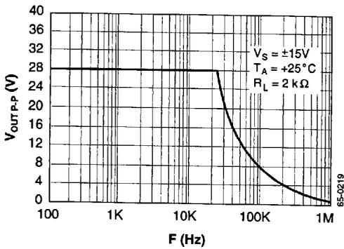
Figure 9. Output Voltage Swing vs. Frequency
