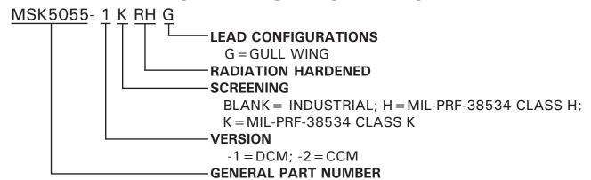
The above example is a DCM, Class K regulator controller with gull wing formed leads.
