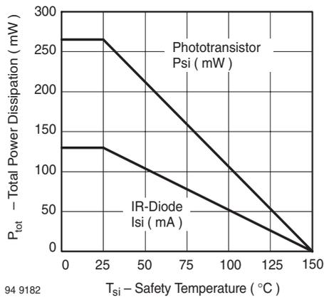
Figure 1. Derating diagram
