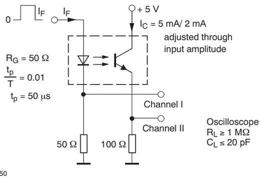
Figure 3. Test circuit, non-saturated operation
