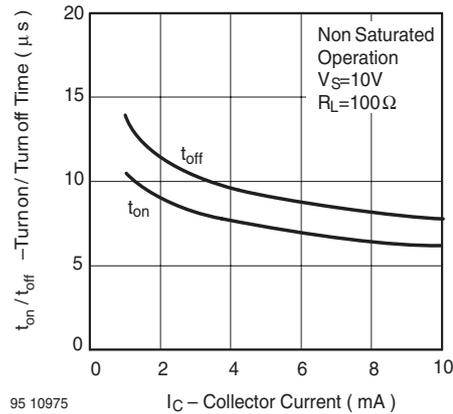
Figure 17. Turn on / off Time vs. Collector Current
