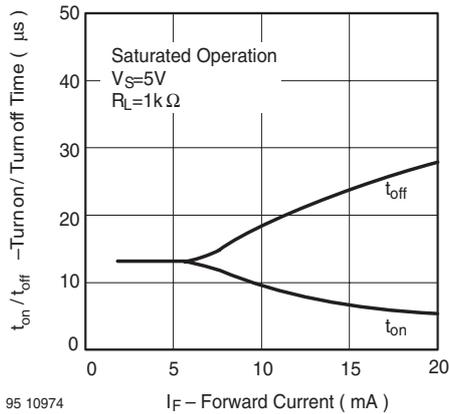
Figure 16. Turn on / off Time vs. Forward Current
